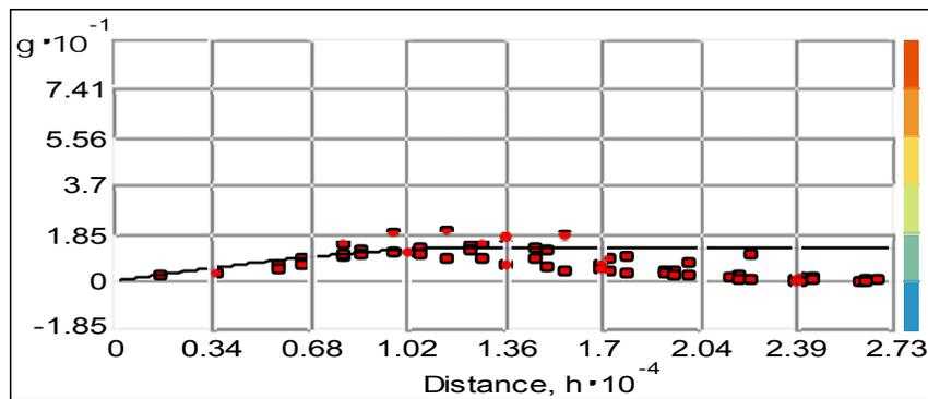
Fig. 6. The semi-variogram model of soil saturated moisture in Farahan region.
